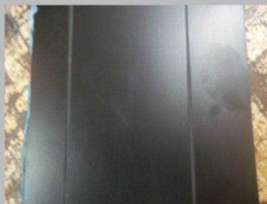
Example of 'V' Grooves that are routed into the PVC sheets to make them easy to bend around bay-poles
